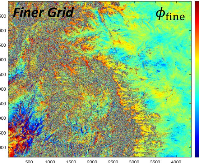
Unwrapping finer-grid phase with the coarser-grid reference
