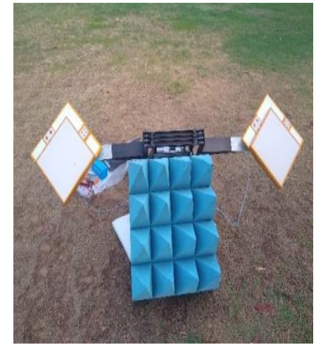
Indigenously developed Wideband Active Radar Calibrator (ARC) (L, S, C & X band)
