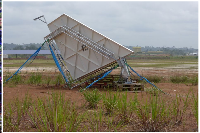
5m trihedral reflector deployed at Nkok near Libreville, on the premises of AGEOS Gabonese Space Agency
