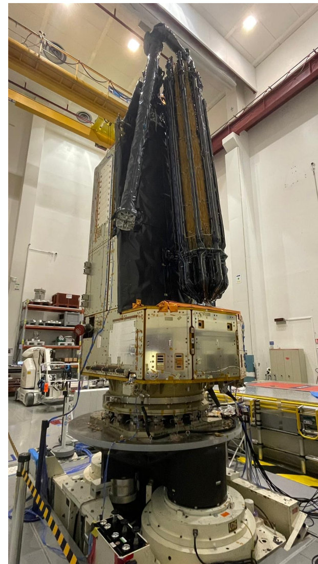
The fully assembled satellite on the shaker in January 2023
