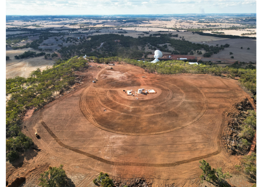
Transponder site – leveled and soil homogenised
